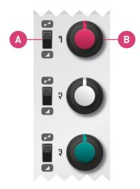
A. Function selector: This switch configures the channel as an attenuator (lower position) or as an attenuverter (upper position).
