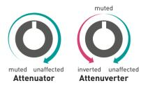
**1. Signal input**. When an input is left unpatched, a constant voltage of +5V (or +10V, as set by the jumper on the back of the module) is sent to the attenuverter or attenuator.
