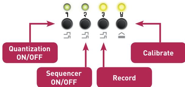
Enable/disable the quantizer or sequencer playback, start sequencer recording, or start the calibration procedure.
