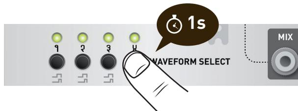
Select a channel by holding the channel selection button for 1 second.
