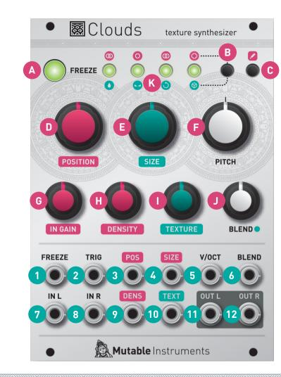
**K. Indicator LEDs.** They work as an input vu-meter (or output meter, when **FREEZE** is active). They can also indicate the quality setting (red), the function assigned to the **BLEND** knob (green), or the value of the four blend-ing parameters (multicolor).
